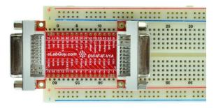
Figure 2: Example of connecting the DVI-IF-IF-V1A on a breadboard (Note: This picture only shows the pins spacing, actual use may not be used on a breadboard)
